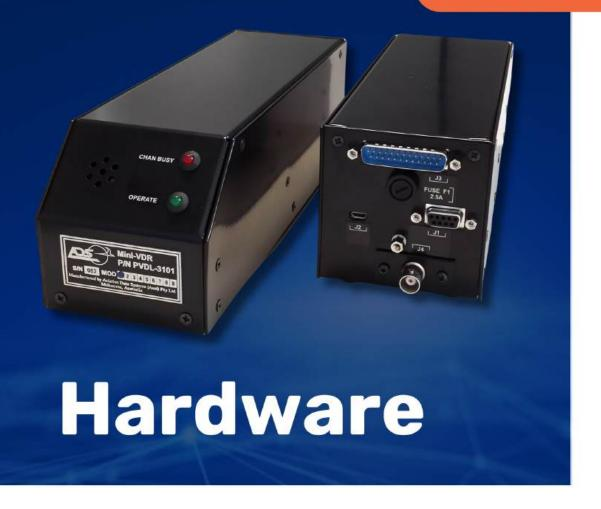
The Mini-VDR is a 50mW signal generator/signal detector-decoder and is a low power realisation of an ARINC 750 VDR. It detects and generates the VHF D8PSK and MSK encoded signals in the range 118.000 to 137.000 Mhz. The Mini-VDR is integrated into the MTP platform and exchanges data via RS-232 or USB to the PVDL software application running on the MTPs integrated notebook PC. The Mini-VDR is powered by 12VDC provided by the MTP platform.
