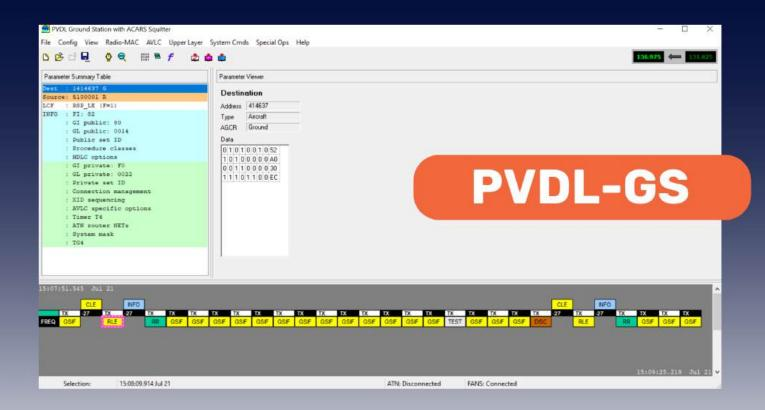
PVDL-GS is the software application that emulates the operation of a VDL Mode 2 ground station. It transmits GSIFs, accepts links with aircraft systems and exchanges data under the control of the VDL Mode 2 protocols as defined by the ICAO SARPS and AEEC 631. It includes a fully integrated A618 protocol engine to support AOA (ACARS-over-AVLC) message handling protocol and conformance.
